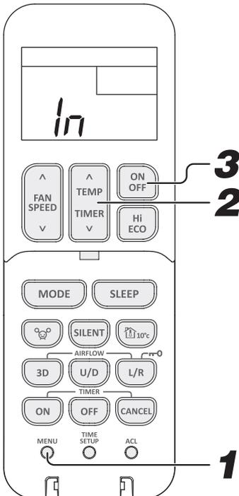
**1** Select the Wireless LAN communication setting by pressing the MENU switch.
