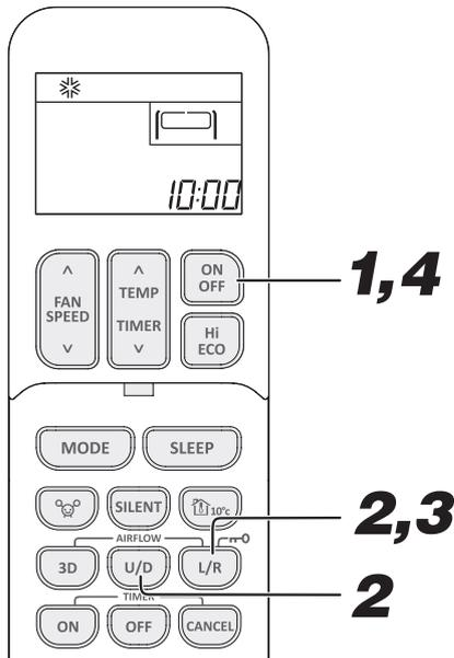
**1** If the air-conditioner is running, press the **ON/OFF** button to stop.
