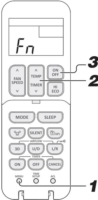
**1** Select the Fan control in heating thermo - OFF by pressing the MENU switch.
