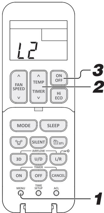
**1** Select the Display brightness adjustment by pressing the MENU switch.
